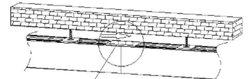
3. When the connector is at the correct position, tighten the screws for the right headrail.
