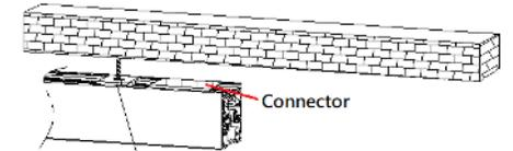
1. Left headrail first. Tighten the screws but not too tight- leave some space for slight adjustment.
