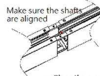
Place the small piece between to make sure the 2 headrails are aligned and then tighten the bolts.
