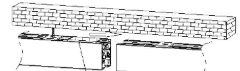
2. Align the right headrail with the left and then slide the connector to where the two headrails meet.
