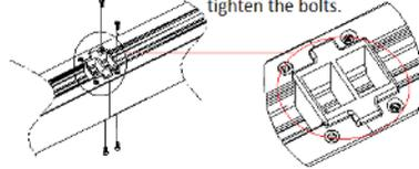
4. Insert the iron sheet into the belt connector.
